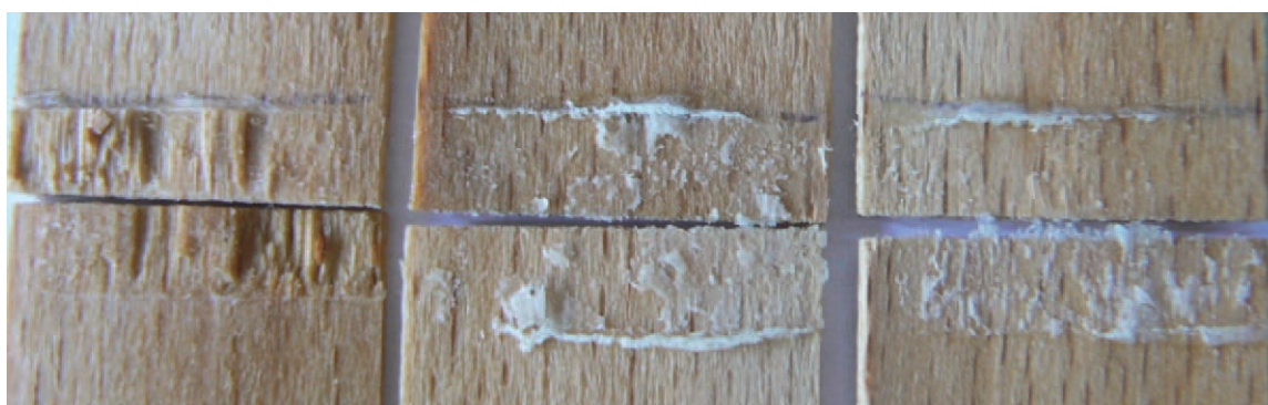
Figure 7 Fractured surfaces (from left) dry glued (a), green glued dried at 20°C (b) and green glued dried at 70°C (c). [Color figure can be viewed in the online issue, which is available at wileyonlinelibrary.com .]
